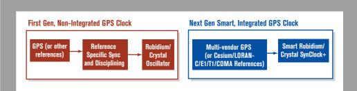
Figure 1. First vs. Next Generation GPS/Multi-Reference Clock designs
